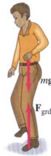
FIGURE 7-12 When the person lands on the ground, the average net force during impact is \bar{F} = F_{\text{grd}} - mg , where F_{\text{grd}} is the force the ground exerts upward on the person.
