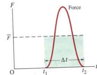
$$F = \frac{\Delta p}{\Delta t} \quad \text{applies to EACH of the objects in a collision}$$
