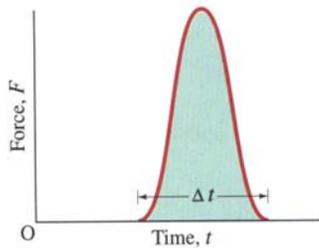
Both particles are deformed in a collision—at the moment of impact,  $F$  jumps from ZERO to a very large value in a very short time and abruptly returns to ZERO again.
